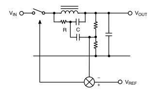
Figure 8. Control Ramp Generated from DCR Inductor Sensing
