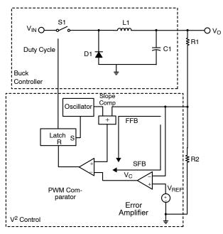
Figure 4. Buck Converter with V2 Control
