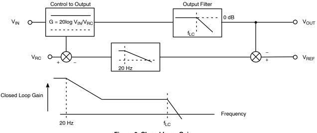
Figure 6. Closed Loop Gain
