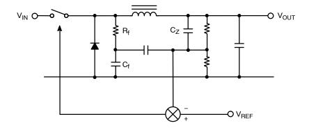
Figure 12. Control Ramp from Voltage Feed Forward
