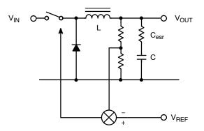
Figure 7. Control Ramp Generated from Output
